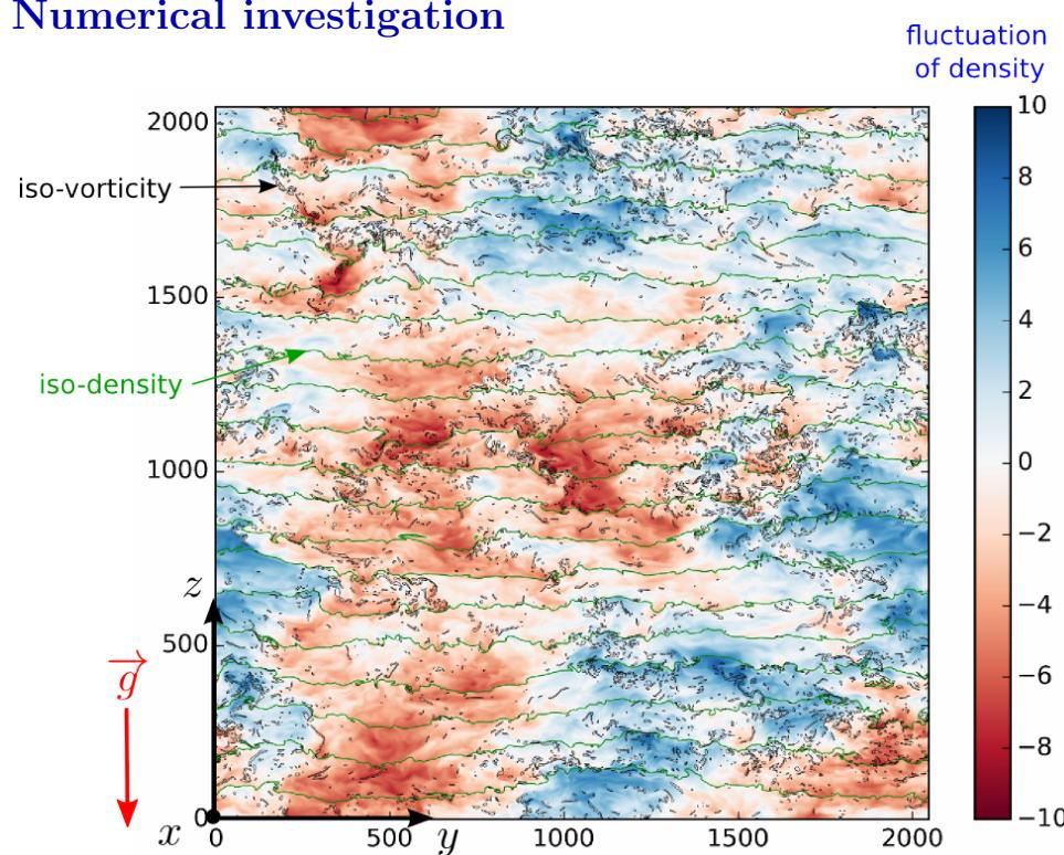
Exemple of numerical simulation : a vertical cut of pure stratified turbulence
